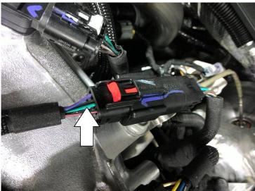
**2019-2025 GM LM2/LZ0** – Remove the front left tire and inner fender liner. Locate the ECU. Remove the black connector and connector cover. Locate the light green wire between the purple wire with a blue stripe and the grey wire with a yellow stripe. Attach the light blue wire here for RPM pickup. Solder the wire and cover with heat shrink for longevity.
