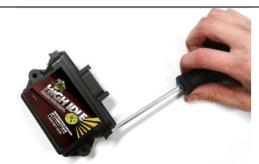
10. For 1998.5-2000 Dodge 24V applications, set "Switch 2" on the circuit board to position 3.
