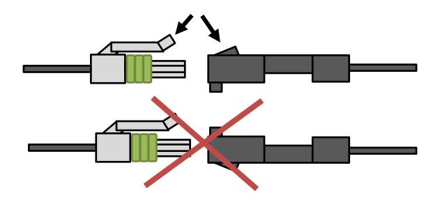
**2003-2004 Dodge 5.9L (CR)** – Locate the engine crankshaft position sensor, located toward the front of the engine on the left side beside the harmonic balancer. Cut off and discard the supplied three pin connector from the blue wire on the BD wiring harness (this is used only up to 2002). Tap the blue wire into the crankshaft sensor wire from pin 3 of the connector. Solder this connection and cover it with heat shrink for longevity.
