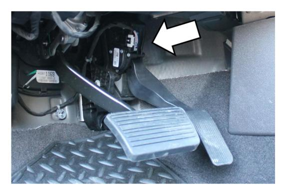
3. Connect the supplied wiring harness to the accelerator pedal position sensor and the other end to the factory wiring harness. Secure the harness with zip ties so that it does not interfere with pedal operation. Removal of the knee bolster may ease installation.
